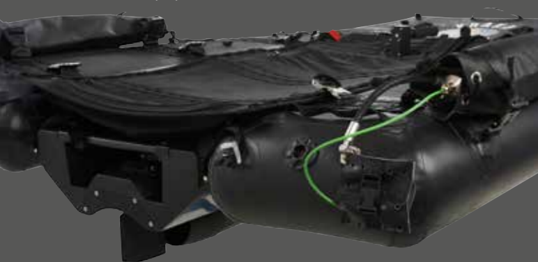
Rapid CO 2 inflation valve, Standard inflation/deflation valve, 13 psi pressure relief valve
